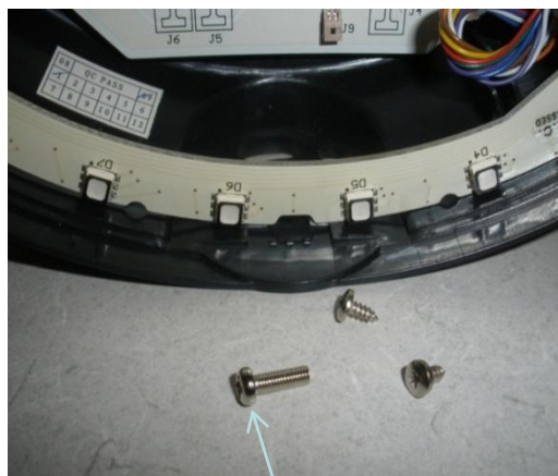
M3 X 10MM PPH SCREW PART OF RGB TOWERLIGHT TOPPER
