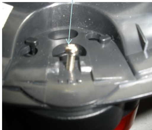
M3 X 10MM PPH SCREW PART OF RGB TOWERLIGHT TOPPER
